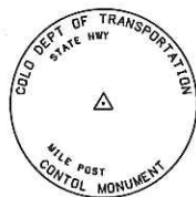
Typical Control Monument Cap Not to Scale
